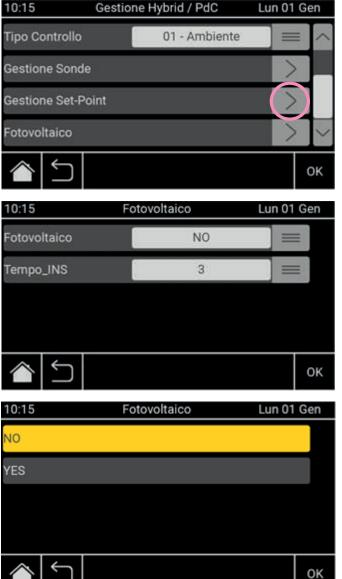
If the photovoltaic check is active, this will be marked by a new icon in Home, indicating whether the ID2 contact is open (no photovoltaic contribution) or closed (presence of photovoltaic contribution).
