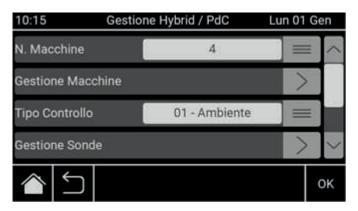
The "Machine Management" menu allows selecting the type of machine connected to the Smart X (Hybrid, HP or Boilers) for each line in the menu. Once the machine type has been selected, Smart X will automatically associate the slave (or slaves, in the case of a Hybrid machine).
