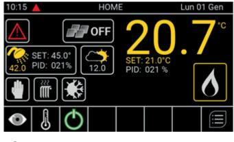
When the HYN goes into cut-off, the icon indicating the external temperature takes on the following configuration:
