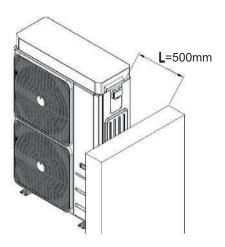
Obstruction or covering of the ventilation openings on the top cover must be avoided.
