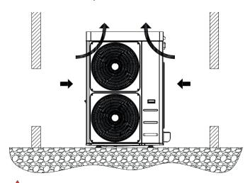
In the case of wind speeds faster than 2.2 m/s, the use of windbreaks is recommended.
