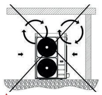
Coverage with roof or positioning near trees or walls is to be avoided in order to prevent air recirculation.
