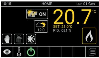
The HOME screen will include the icon for the domestic hot water production control (if present), which will show the temperature reading, setpoint and PID calculation.
