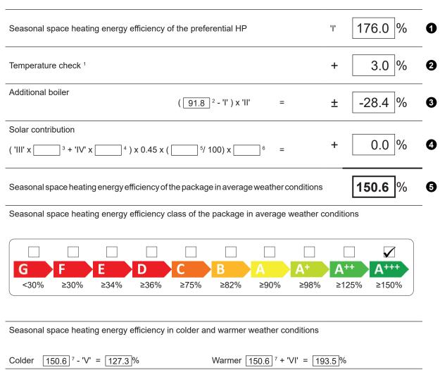
The energy efficiency of the package of products provided for in this sheet may not correspond to its actual energy efficiency once installed in a building, as the efficiency is influenced by further factors such as the heat loss in the distribution system and the dimension of the products in relation to building size and characteristics
