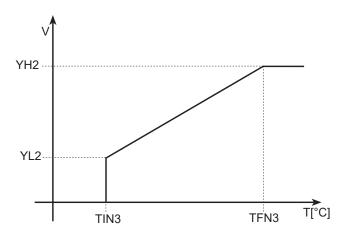
During operation in heating mode, the value of 0-10V signal sent to the fan heater depends of the reading of AQUAPUMP water delivery temperature probe (NTC3 probe - HYN delivery probe) and varies linearly between the minimum voltage value (par. YL2) at the temperature corresponding to the minimum speed (par. TIN3) and the maximum voltage value (par. YH2) at the temperature corresponding to the maximum speed (par. TFN3) as described in the graph below.
