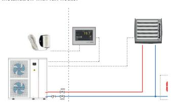
This type of system must be selected to use AQUAPUMP HYBRID together with one or more fan heaters code ABXXXIT-HY. This programming is to be made:
