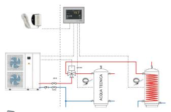
The Smart X NTC1 probe must be placed inside the heating tank.
