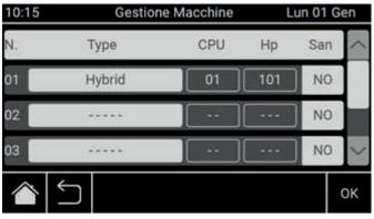
The Smart X will automatically associate the two addresses 01 to the CPU and 101 to the heat pump. The allocation of heat pump address 101 must be chosen manually on the heat pump LCD panel.
