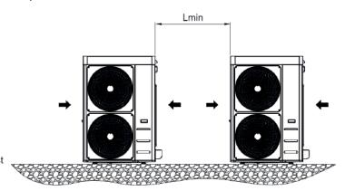
In the case of side-by-side units, the minimum distance Lmin to be observed between them is 1 m.
