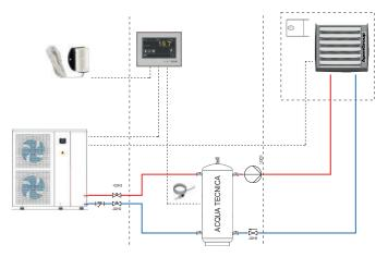
This type of system must be selected to use AQUAPUMP HYBRID together with a technical water tank, a hydraulic separator or a reservoir.
