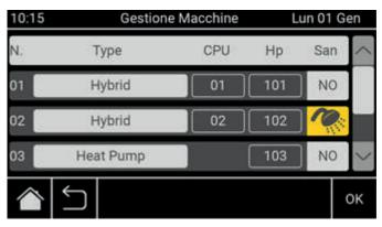
By pressing the button under the "San" column, you can enable DHW check management for that specific machine. The "San" button will change from grey with the word "NO" to yellow with the shower symbol, indicating that the check has been activated. DHW check can be activated for one or more machines simultaneously.
