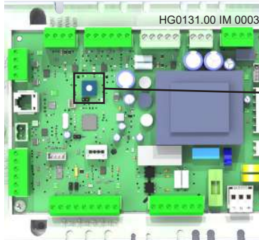
Switch for CPU PCB address
